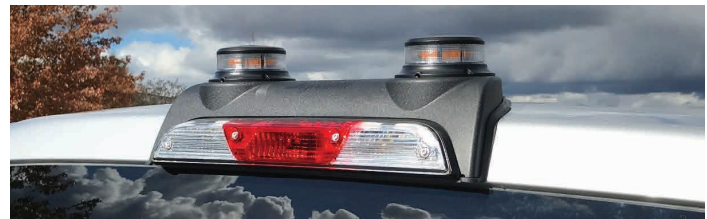
Installed into factory third brake light (amber beacons)
