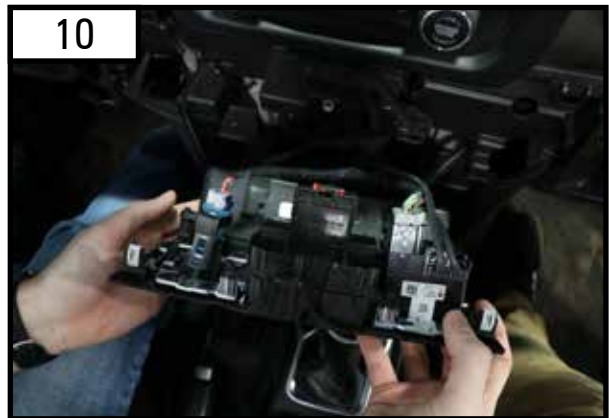
Pry out the window control panel from the top using the plastic trim removal tool and work your way down.
