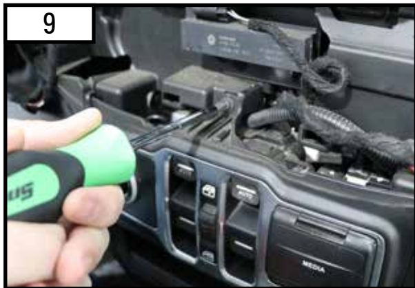
Remove the screw using a #2 Phillips head screw driver.
