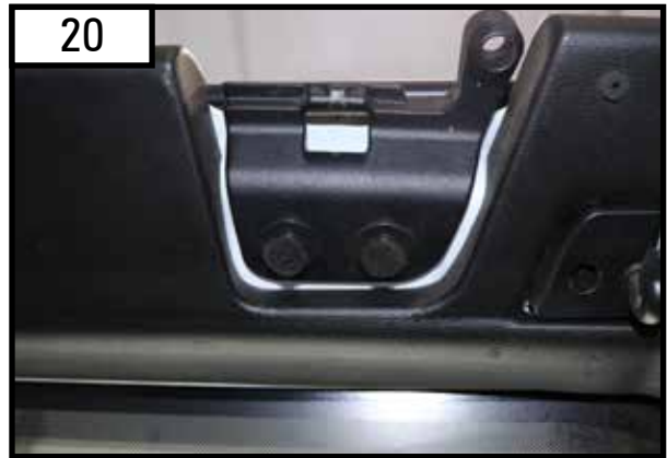
Unlatch and open the soft top or remove the hard top front panels. Remove the felt padding on top of the bolts holding in the bracket.
