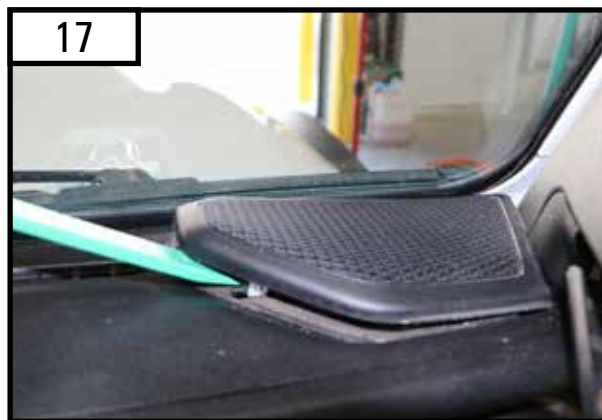
17 Use the plastic trim removal tool, to pop off the speaker cover on the passenger side.
