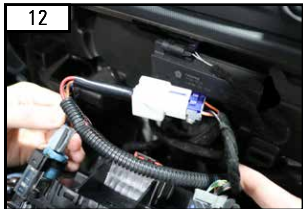
Connect the white connector of the jumper power harness to the original plug you just disconnected in STEP 11. Connect the grey connector back in to the 12v socket
