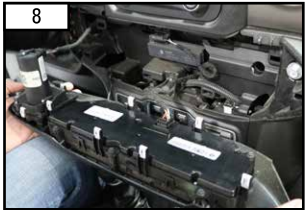
Disconnect the two connectors attached to the center dash control system and then set the unit aside.
