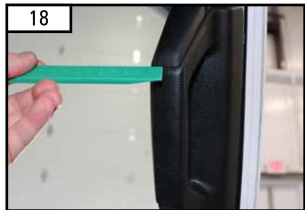
18 Using the plastic trim removal tool, pop off the two bolt covers for the A-pillar trim piece
