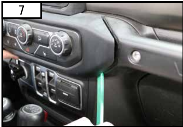
Using a plastic trim removal tool, pry off the center dash control system by starting on the outside and working your way around.
