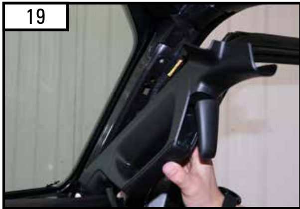
Remove the two bolts with a 10mm socket, once bolts are removed pop off the trim panel.
