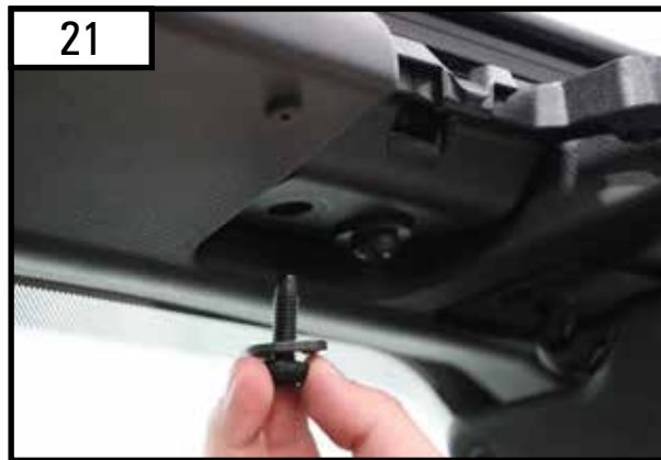
Remove the two bolts per side using a T-40 Torx socket, and pull the bolts out all the way.
