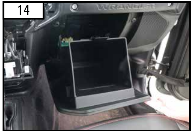
14 The glove box will need to be removed from the vehicle. Pull the back of the glove box towards you and then tilt the glove box down to remove.
