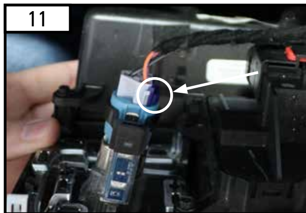
Tilt the window control panel out so you can access the 12v socket connection. Push the blue tab in and pull out the connector.
