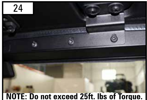
Before the bolt are completely tightened down you will need to push up on the shroud to ensure a good seal along the windshield. *Repeat steps 23-24 for driver side installation.
