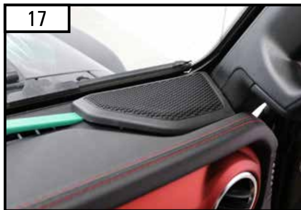
17 Use the plastic removal trim tool to pop off the speaker cover on the passenger side and set aside.
