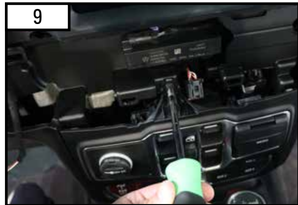
Remove the screw using a No. 2 Phillips head screw driver.
