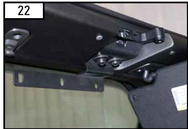
(Passenger side shown) Take the bracket provided and install on top of the hard top bracket. When re-installing the two T-40 Torx bolts make sure to leave the bracket loose with adjustability forward and backwards. Repeat steps 20-22 for Driver side bracket installation.
