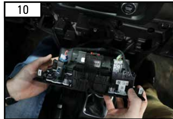
Pry out the window control panel using the plastic trim removal tool and start from the top and work your way down.
