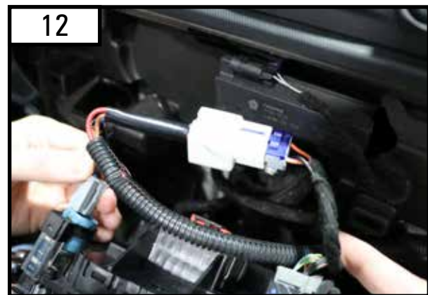
Connect the White connector to the original plug you just disconnected in STEP 11. Connect the grey connector back into the 12v socket
