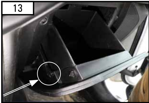
13 Open up the glove box and disconnect the strut by pulling up and out.
