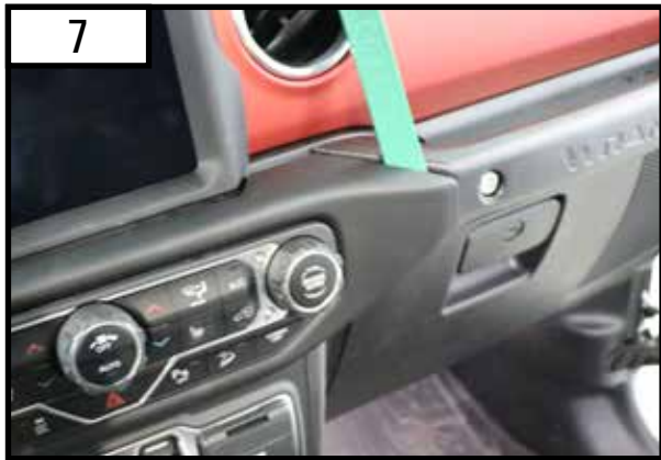
Using the plastic trim removal tool, pry off the center dash control system by starting on the outside and working your way around.
